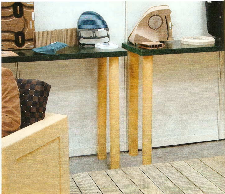
At the Ligna-Fair 2005 in Hannover (Germany) a variety of wood plastic composites (WPC) was shown including armchairs, tables, automotive parts and outdoor flooring. Wood flour is replacing plastics and/or timber.
