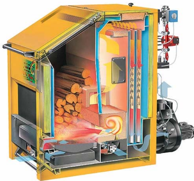
Figure 3: Modern wood gasifier boiler (Source: www.koeb-schaefer.com )
